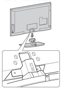
3 Fix the TV to the stand according to the arrow marks ★ that guide the screw holes using the supplied screws.
